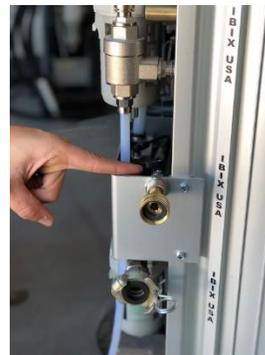
**Testing System Pressure** – The last step required on the IBIX Maintenance Checklist is testing the system air pressure. Each system has a minimum CFM (Cubic Feet per Minute) requirement. Please see the Multi-System Spec Sheet for system CFM requirements.
